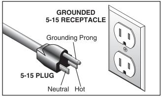
Figure 2. Typical 5-15 plug and receptacle.
